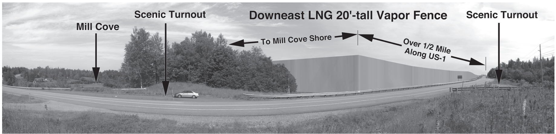
Vapor fence simulation based on Downeast LNG's 23 May 2012 filing to the Federal Energy Regulatory Commission (FERC) about safety hazards resulting from an LNG release at their proposed site. © 2012 SPB
