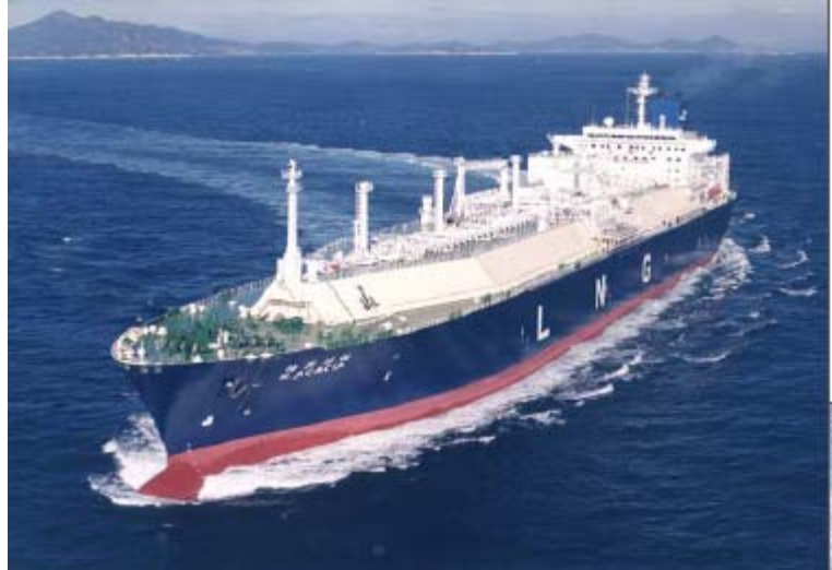
LNG Vessel with Membrane Tanks
